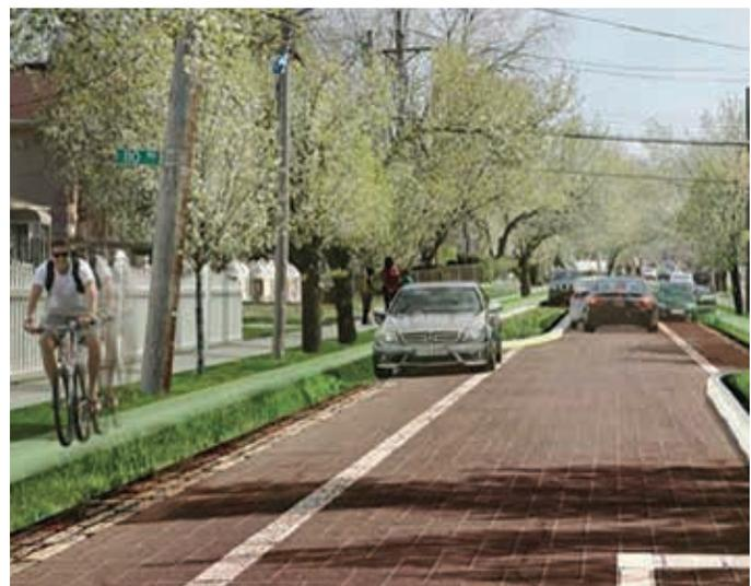
In Flushing, New York, a cloudburst street combines permeable pavement and green infrastructure to capture runoff.
